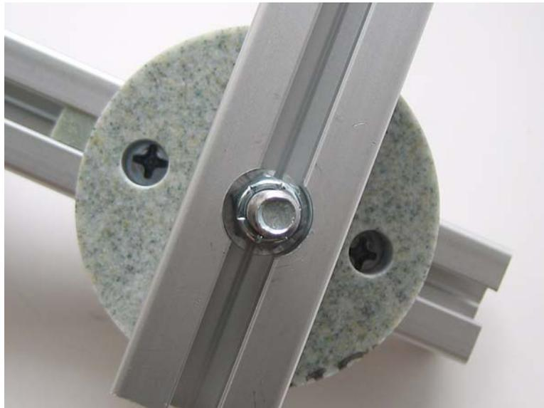
*Fig 11: Access holes for adjusting the camera support arm length.*
