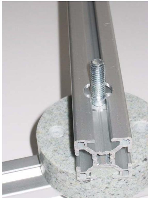
*Fig 3: Pivot bolt/stud showing unthreaded section.*
