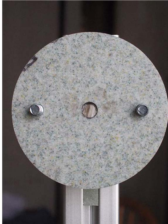
*Fig 6: Head of the bolt cut off and epoxied into the bearing pad.*
