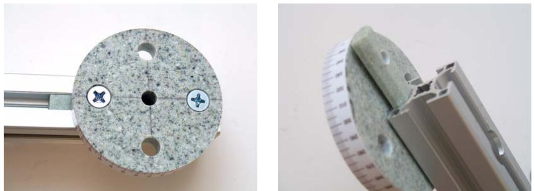
*Fig 9: Countersunk screws and attaching to frame with t-nuts*
