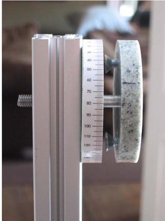
*Fig 8: Bolt passing through bearing pads and framing and flat head screws.*
