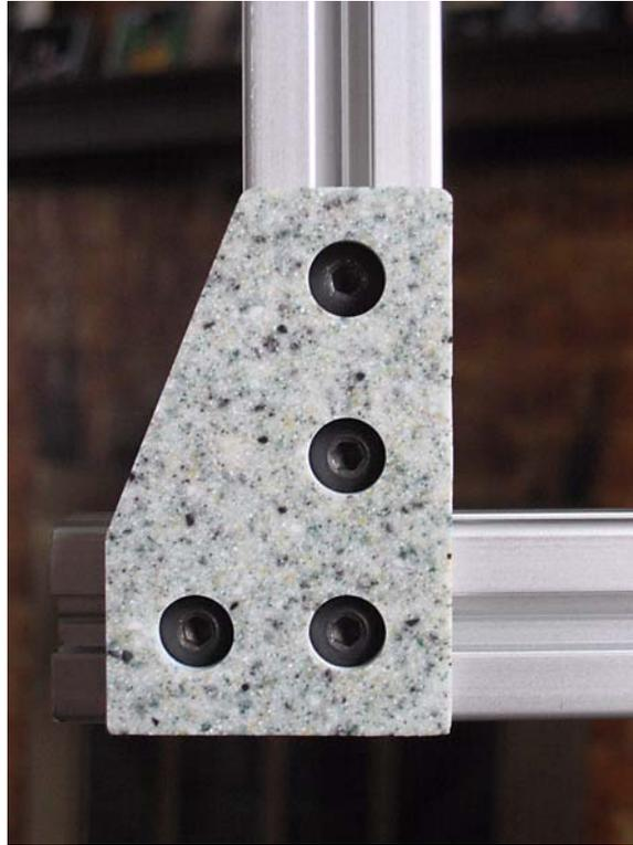
*Fig 4: Joining plate made from 1/2 inch corian.*
