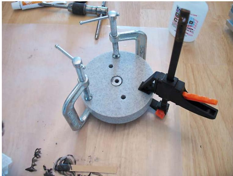
*Fig 19: Gluing and clamping two discs together. Note the 1/4-20 tripod socket.*
