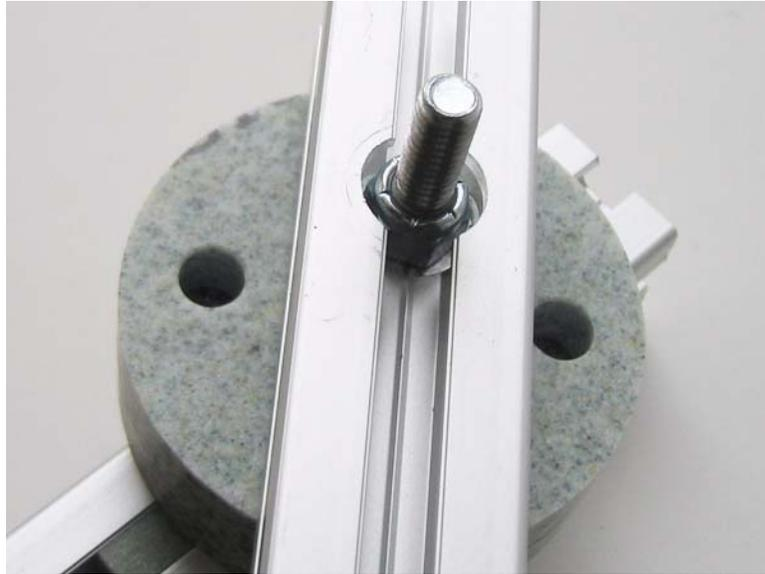
*Fig 7: The nylon stop nut which keeps the joint together.*
