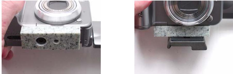
*Fig 15: Camera mount to offset the tripod socket.*
