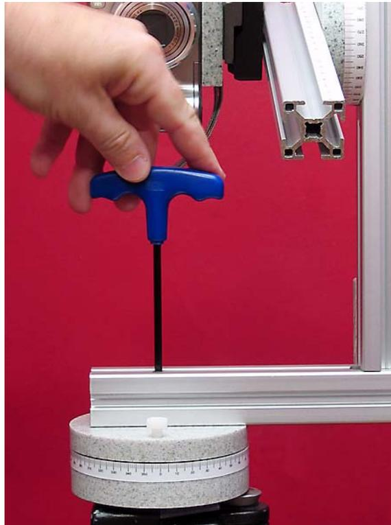
*Fig 20: Adjusting the shoulder screw in the rotating base.*
