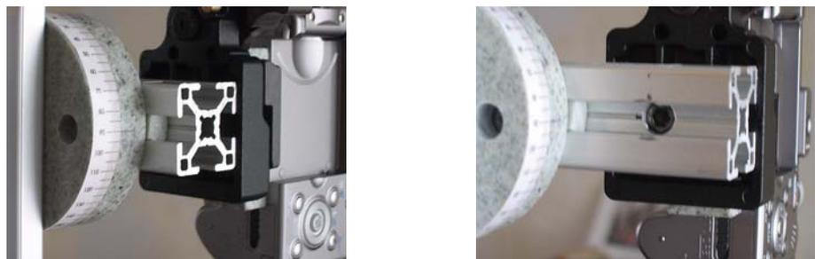
*Fig 14: Countersinking the Quickmount bolt to allow additional travel of the camera support arm.*
